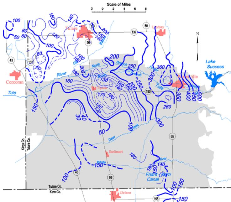
Figure D-1. Lines of Equal Elevation of Water in Wells, Unconfined Aquifer (Spring 2010)
